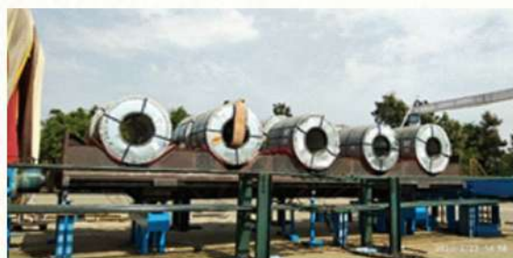
Wagon body loaded with coils for Squeeze Load Test
