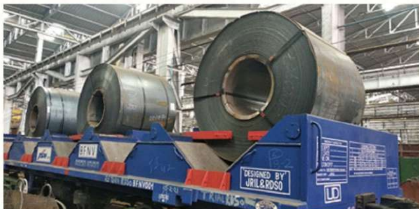
Wagon-BFNW001 loaded with coils for Oscillation trials
