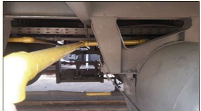
Additional Water over flow provide with elbow for water jet downward to earth.
