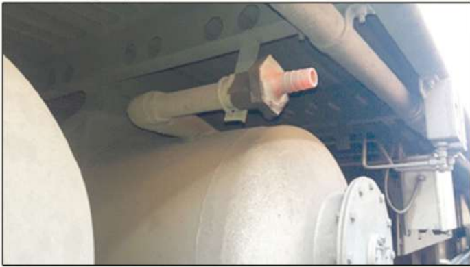
Existing Water filling /Overflow Pipe
