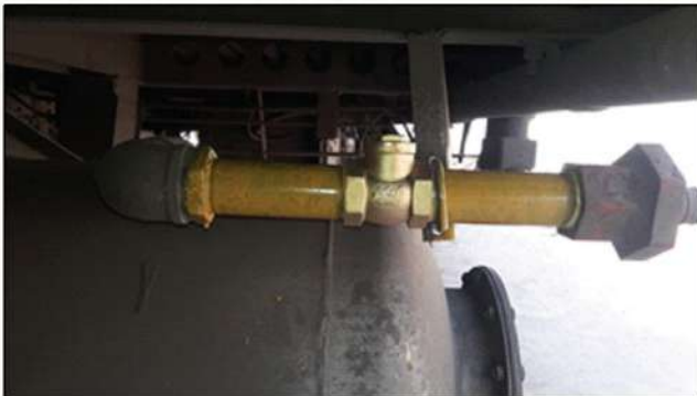
Additional Non-Return Valve Provide on Both water filling /overflow pipe line.
